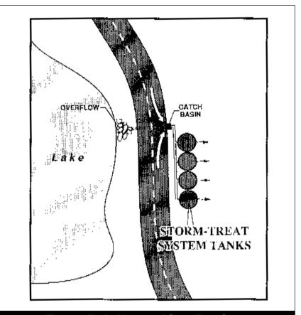
Figure 1: Typical Layout of StormTreat System
