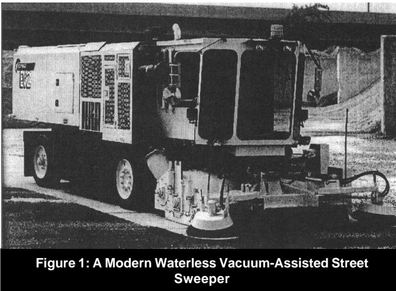
Figure 1: A Modern Waterless Vacuum-Assisted Street Sweeper
